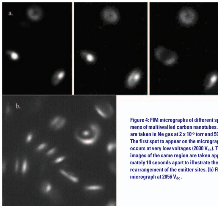
**Figure 4:** FIM micrographs of different specimens of multiwalled carbon nanotubes. Images are taken in Ne gas at  $2 \times 10^{-5}$  torr and 50 K. (a) The first spot to appear on the micrograph occurs at very low voltages (2030  $V_{dc}$ ). Three images of the same region are taken approximately 10 seconds apart to illustrate the rearrangement of the emitter sites. (b) FIM micrograph at 2056  $V_{dc}$ .
