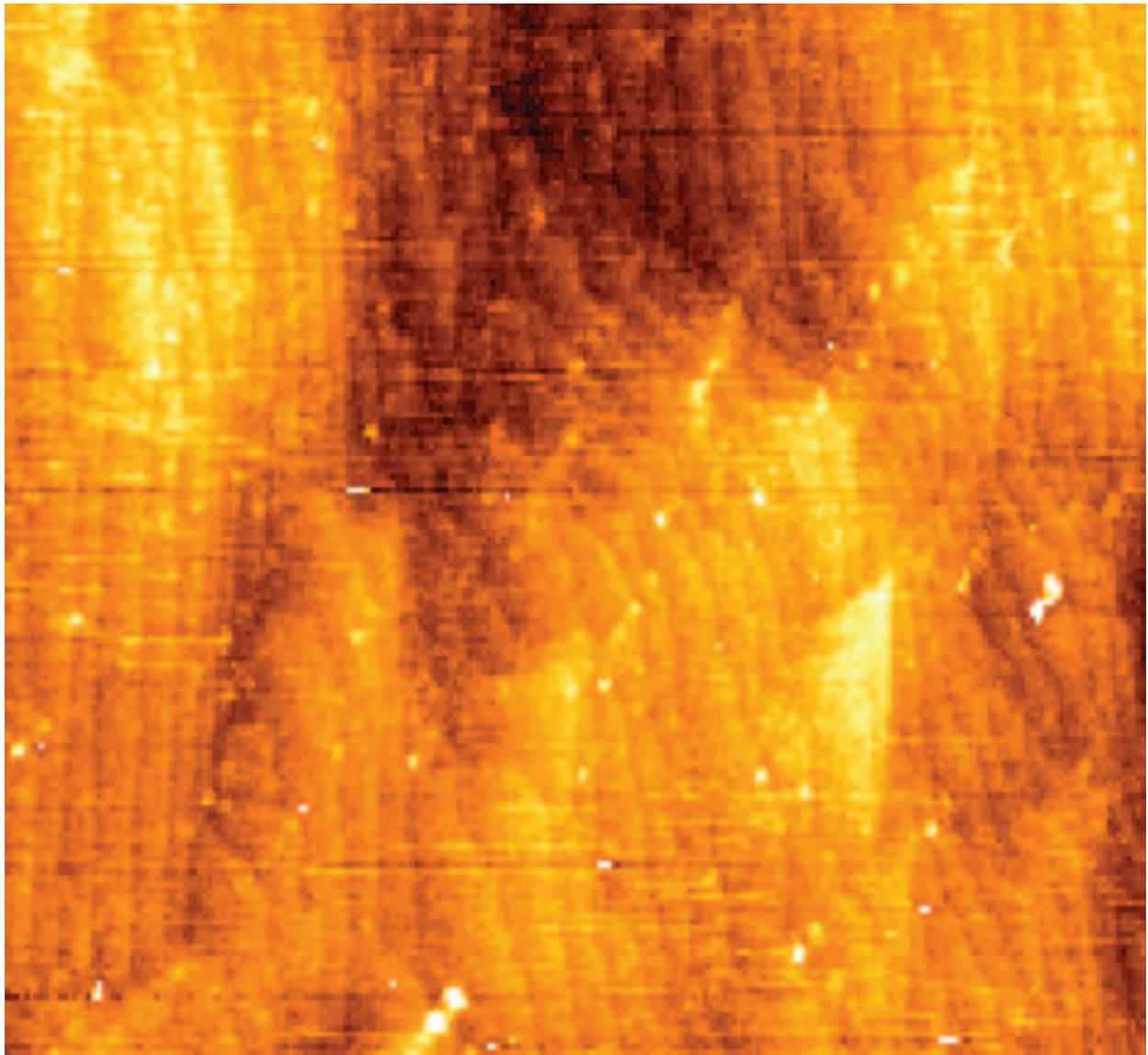
**Figure 2: AFM image (3 micron scan) of a H-passivated Si surface. Identical to image of sample with UDAME monolayer.**
