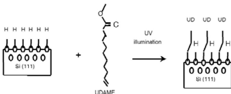
**Figure 1: Attachment of a UDAME monolayer on a Si(111) surface. Note that the UDAME molecule is too large to occupy every H-Si position, which means 100% film coverage is not possible.**
