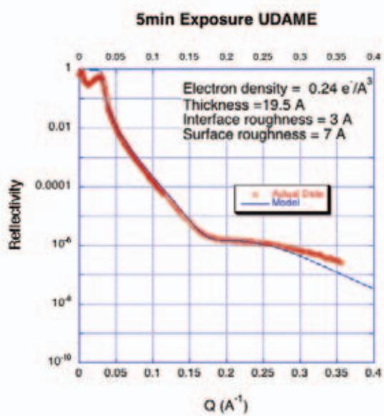
Figure 4: X-ray reflectivity spectra of five-minute exposed sample.
