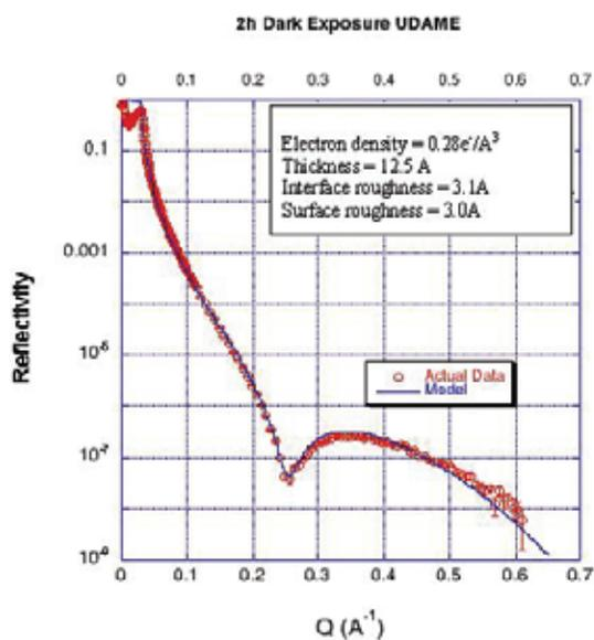
Figure 3: X-ray reflectivity spectra of two-hour dark exposed sample.
