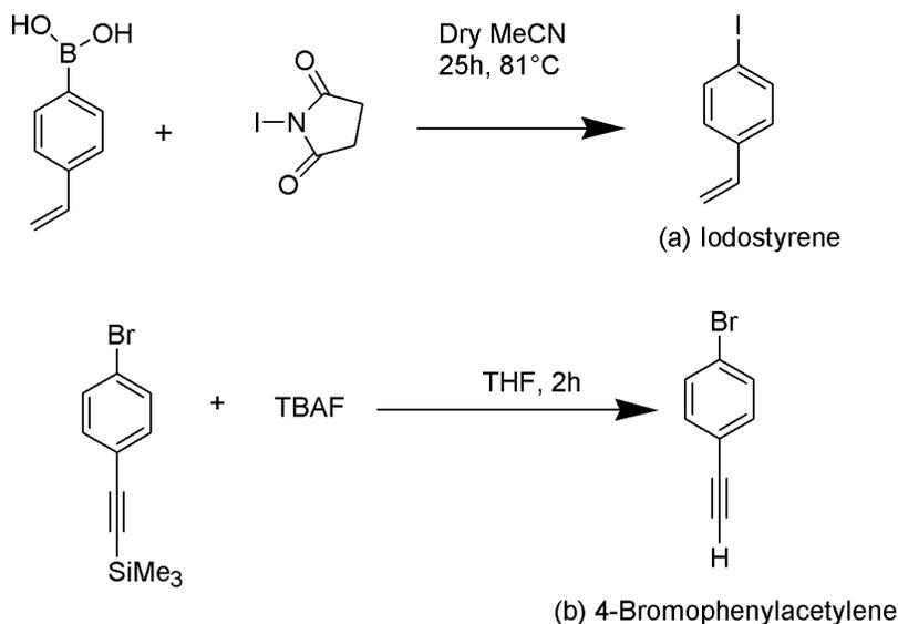
Figure 3: Synthetic schemes for (a) iodostyrene and (b) 4-bromophenylacetylene.
