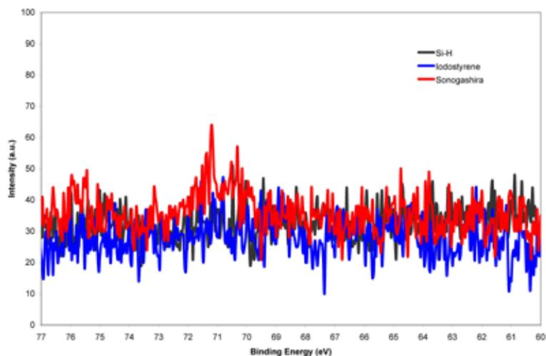
Figure 8: XPS detailed scans of Br3d binding energy.
