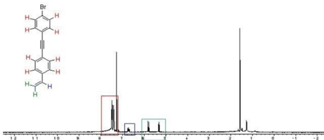
Figure 5: NMR spectrum of 4-(4-Bromophenethynyl)styrene prepared by a wet chemical Sonogashira reaction.
