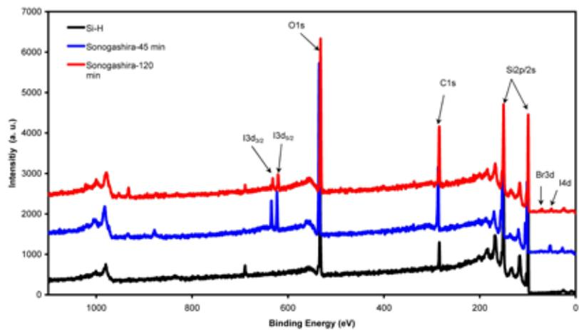
Figure 9: XPS general scans comparing a Si-H wafer (black), a wafer that underwent UV irradiation in the presence of iodostyrene and then 45min of Sonogashira coupling (blue), and a wafer that underwent UV irradiation in the presence of iodostyrene and then 120min of Sonogashira coupling (red).
