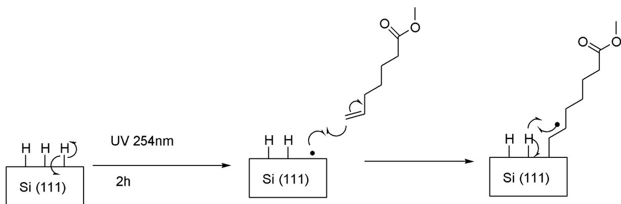
**Figure 1: Radical mechanism used to create self-assembled monolayers.**
