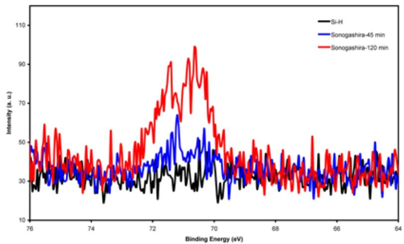
Figure 10: XPS detailed scans of Br3d binding energy.
