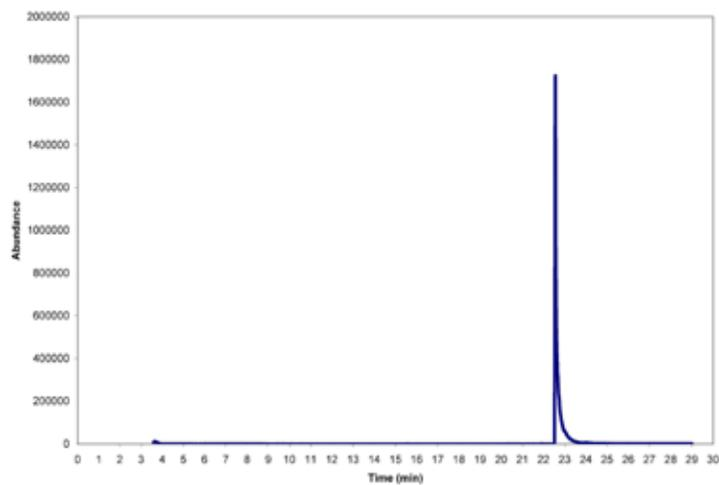
**Figure 6: GC-MS data for the solution phase Sonogashira coupling confirming synthesis of 4-(4-bromophenethynyl)styrene.**
