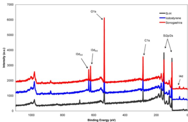
Figure 7: XPS general scans showing a hydrogen-passivated silicon wafer (black), a HPS wafer that had been UV-irradiated in the presence of iodostyrene (blue), and an HPS wafer that was UV-irradiated in the presence of iodostyrene and then subjected to a Sonogashira coupling reaction with 4-bromophenylacetylene (red).
