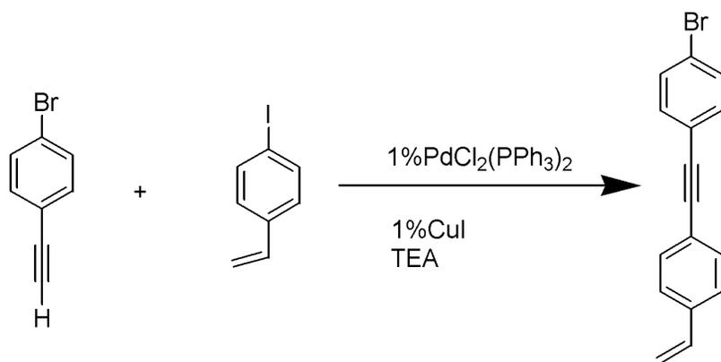
Figure 2: Synthetic scheme for wet chemical Sonogashira coupling.
