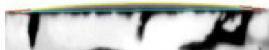
Figure 6. Sessile drop of water on a glass microscope slide that has been cleaned with Nochromix for 1 hr, sonicated in methanol for 15 min, and plasma-cleaned in O 2 for 30 sec. The contact angle is 4°, indicating a clean and hydrophilic surface.
