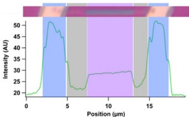
**Figure 5.** A profile of green reflected intensity along the longitudinal axis of the nanowire and its contacts. The data are from the red-green-blue optical microscope image that is aligned above. The Ni contacts,  $\text{Ni}_x\text{Si}_y$ , and Si channel are indicated by the blue, gray, and purple shaded regions, respectively.
