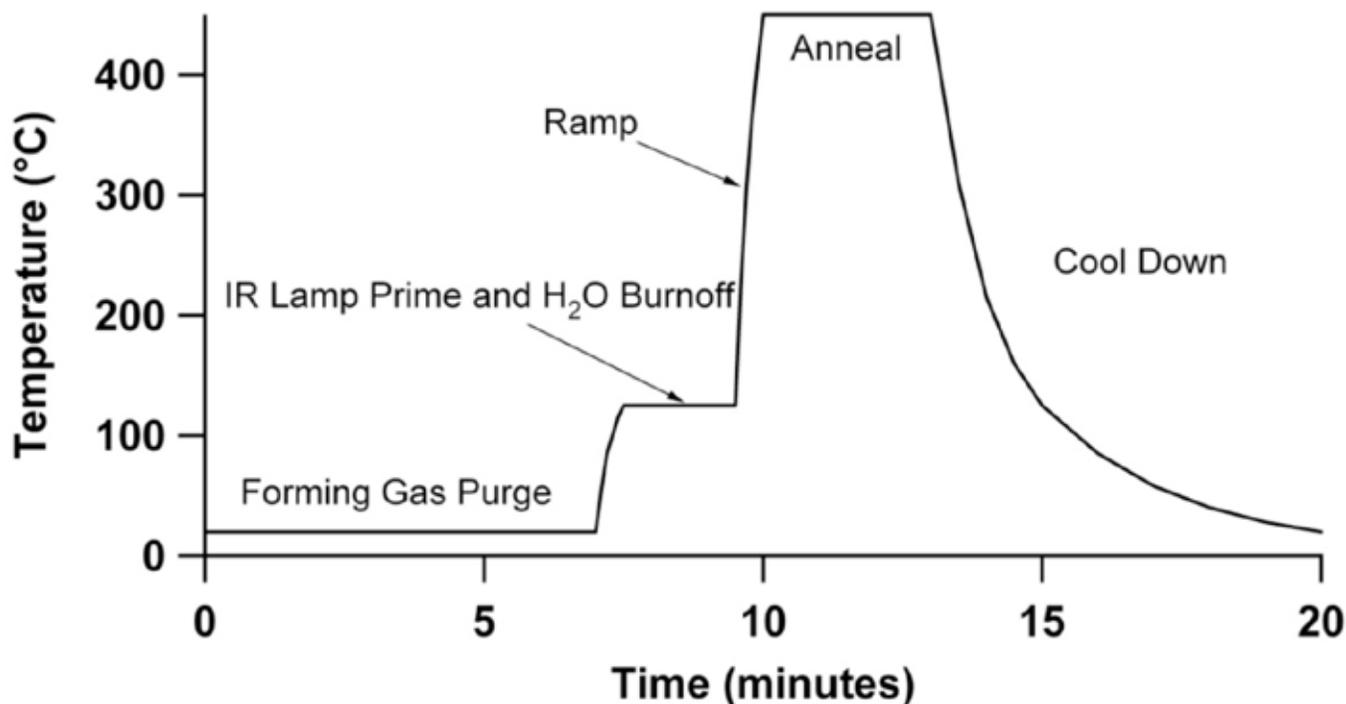
**Figure 2.** Temperature as a function of time during a rapid thermal anneal. In this example, the sample spends 3 min at the 450° C annealing temperature. The process quickly ramps to the anneal temperature in order to minimize the time spent at intermediate temperatures.
