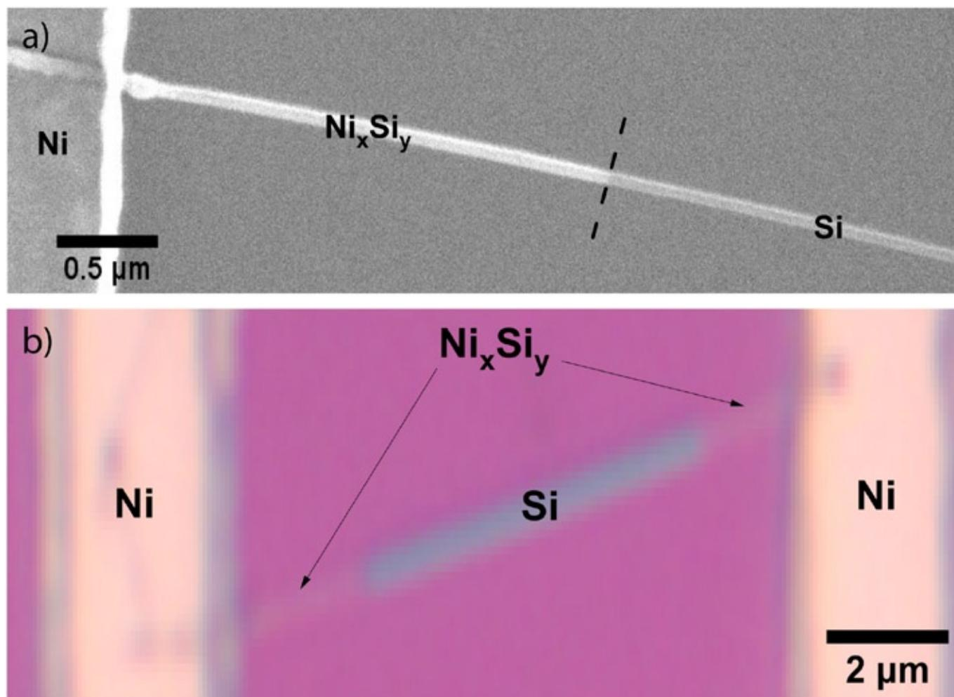
**Figure 3.** (a) A scanning electron microscope image of a silicon nanowire contacted lithographically with Ni and then annealed to form a  $\text{Ni}_x\text{Si}_y$ -Si heterostructure. The dotted line is a guide to the eyes. (b) An optical microscope image of a Si nanowire implemented as a field effect transistor with  $\text{Ni}_x\text{Si}_y$ -Si heterostructures as contacts.
