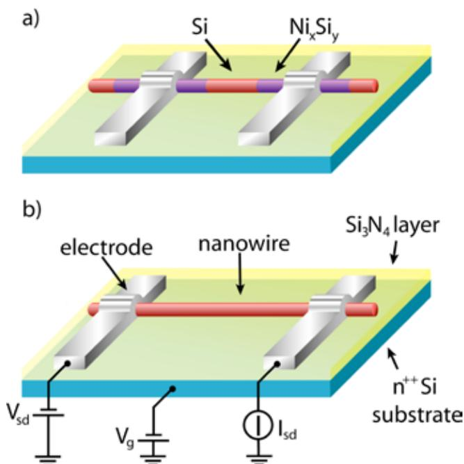
**Figure 1.** (a) Schematic of a Si nanowire (red), Ni electrodes (silver), and  $\text{Ni}_x\text{Si}_y$  segments (purple). (b) Schematic of a nanowire field effect transistor. Source-drain voltage, gate voltage, and source-drain current are  $V_{sd}$ ,  $V_g$ , and  $I_{sd}$ , respectively.
