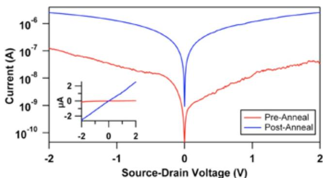
**Figure 4.** A semi-log plot of current as a function of source-drain voltage for a representative silicon nanowire FET. The pre- and post-anneal curves are shown in red and blue, respectively. After annealing, the contact resistance decreases and the behavior becomes ohmic. The inset shows the linearly scaled plot.
