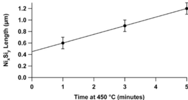
**Figure 6.**  $\text{Ni}_x\text{Si}_y$  length as a function of time at 450 °C.
