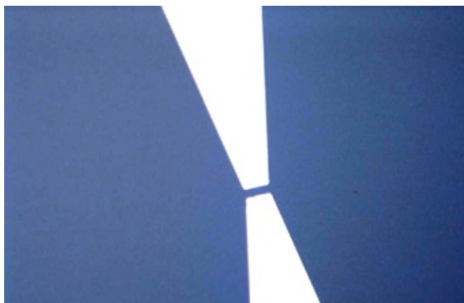
Figure 11. Pt electrodes sputtered on top of ZnO thin film, showing a clean shape and gap of about 10 \mu\text{m} between electrode pairs.
